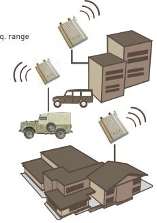
**Note:** The area covered depends upon the outside signal strength. The Shireen Single band Cellular Repeater/Amplifier is designed considering -75dB as the available signal strength. As outside signal strength decreases, coverage area decreases. For poor outside signal areas or for increased interior coverage, use a directional antenna.
